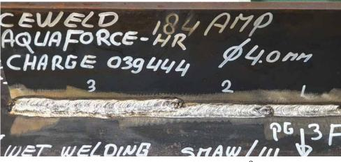
Fillet weld vertical down (PG / 3Fd) in 1 2 3 layers
