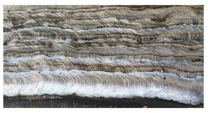
Macro of a pure weld metal without pores
