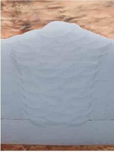
Cover layers with fine scaled seam surface without porosity or inclusions
