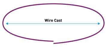
Cast - The cast of welding wire is essentially the diameter of the wire when you take it off of the spool. Average weld wire packaged on a spool has a cast of 660 mm whereas a true robotic weld wire does not have cast, but instead forms a sinewave when laid on the floor. This permits a faster welding speed and less spatterbecause the weld wire is precisely melted into the joint.
